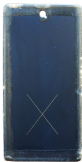
SermeTel Blue on low-carbon steel after 7000 hours of Salt Spray test
