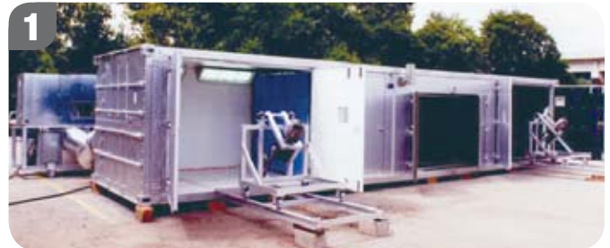
This mobile workshop is shipped and packaged as two independent containers. The workshop is useful for loose axial compressor diaphragms, bladed wheels and centrifugal compressor diaphragms. The units include an oven, a blasting/burnishing cabinet and a spray booth area.
