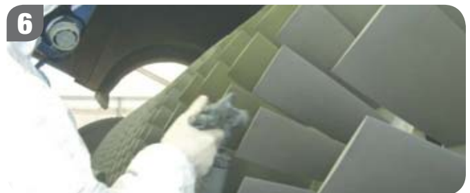
Humidity control is essential for applying a smooth, uniform base coat. Base coat materials are filled with atomized aluminum pigment, which creates rough, coarse overspray if applied at incorrect humidity values.
