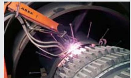
Applying a customized surface coating to the "fir tree roots" section of the turbine disk improves both structural integrity and blade stability. The improved stability prevents "bucket rock," which is often found in gas turbines used for standby or peaking service.
